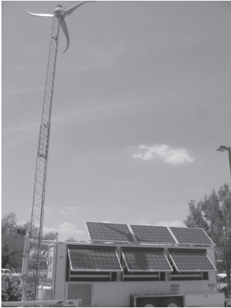
Mobile Gen's Mobile Trailer serves as a portable power/water treatment plant in support of first responders, disaster relief and rebuilding operations.
